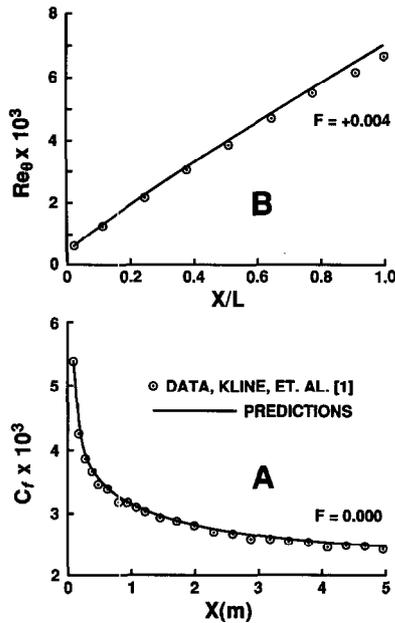
Fig. 1. Predictions compared to data. (A)  $F = 0.00$ ,  $u_s = \text{constant}$ . (B)  $F = +0.004$ ,  $u_s = \text{constant}$ .  $L = 2.286 \text{ m}$  (7.5 feet).
