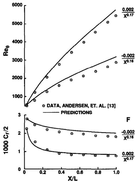
Fig. 5. Predictions compared to data.  $F \sim x^{-0.17}$ ,  $u_s \sim x^{-0.15}$ ,  $F \sim x^{-0.16}$ ,  $u_s \sim x^{-0.20}$ .  $L = 2.286$  m (7.5 feet).
