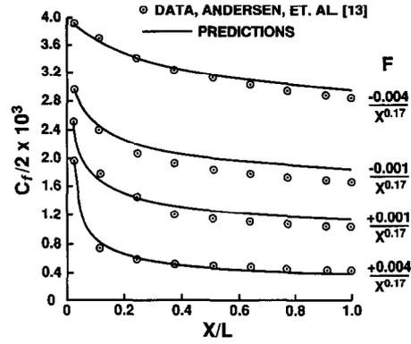
Fig. 4. Predicted skin friction compared to data.  $u_s \sim x^{-0.15}$ ,  $L = 2.286$  m (7.5 feet).
