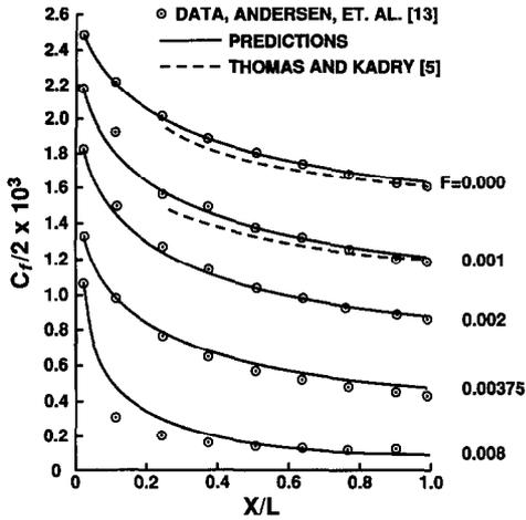
Fig. 3. Predicted skin friction compared to data.  $u_s =$  constant.  $L = 2.286$  m (7.5 feet).
