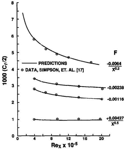
Fig. 6. Predicted skin friction compared to data.  $u_s = \text{constant}$ .
