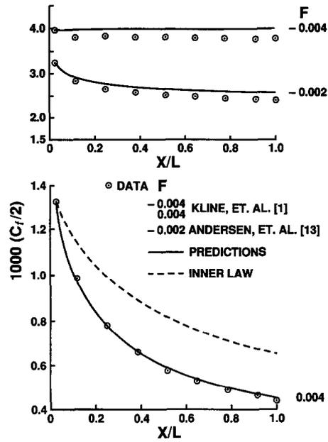
Fig. 2. Predicted skin friction compared to data.  $F = +0.004$ ,  $u_s = \text{constant}$ ;  $F = -0.002, -0.004$ ,  $u_s \sim x^{-0.15}$ .  $L = 2.286 \text{ m}$  (7.5 feet).
