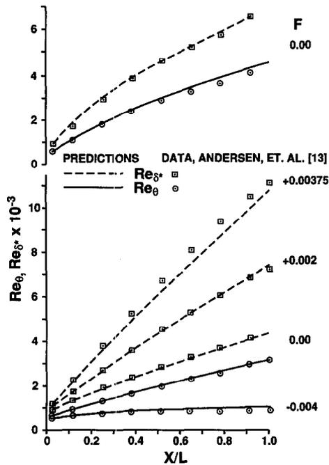
Fig. 7. Predicted momentum and displacement thickness Reynolds numbers compared to data.  $F = 0.00$ ,  $u_s \sim x^{-0.20}$ ;  $F = 0.00375$ ,  $0.002$  and  $0.00$ ,  $u_s = \text{constant}$ ;  $F = -0.004$ ,  $u_s \sim x^{-0.5}$ .  $L = 2.286$  m (7.5 feet).
